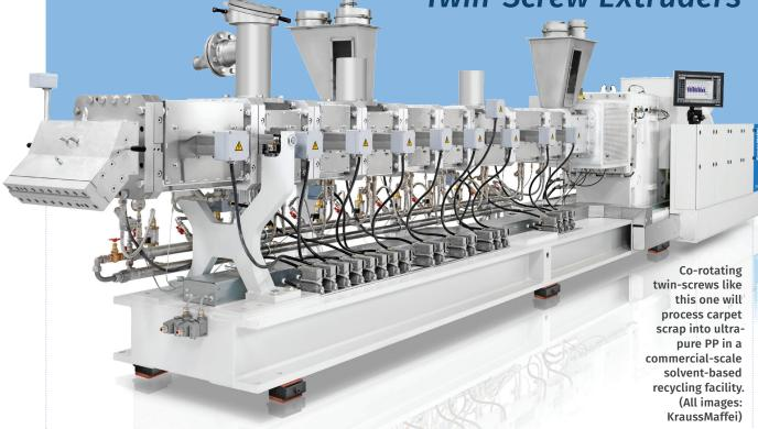
Just now being applied commercially, solvent-based recycling turns colored polyolefin waste into clear, clean and even food-grade resin comparable to virgin—all while keeping the polymer structure intact. Specially engineered systems of tandem twinscrew or twin- and single-screw extruders can do the trick.
