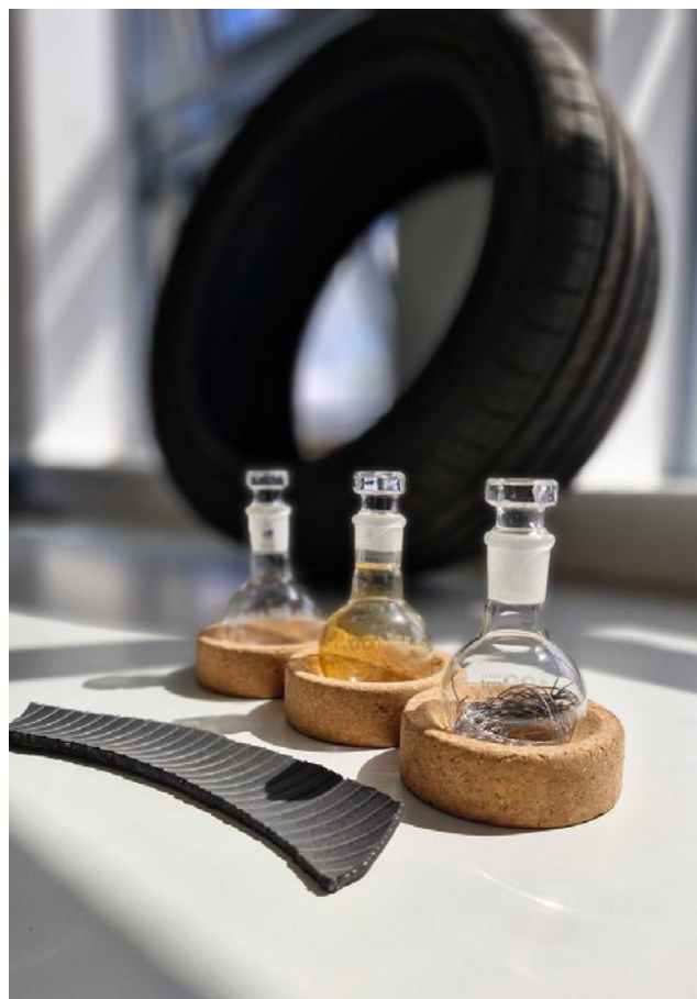
The OxyCycle process can separate waste tyres into its constituent parts, rubber, carbon black, and textiles.
