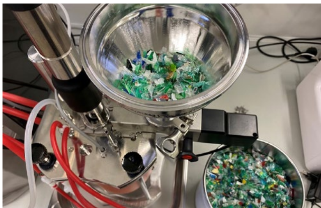
Laboratory reactor for enzymatic plastic degradation.
