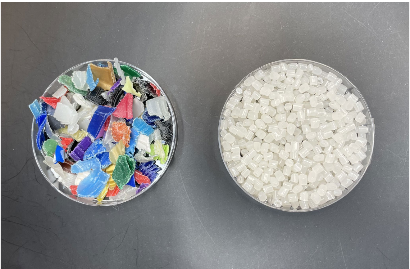
Bottle cap plastic purified by Reventas to produce virgin-like recycled plastic
